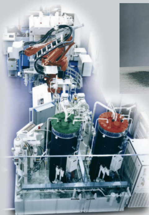
Professionally manufactured cover plate. A robot applies the reaction mixture (glass fibre/PU) with the utmost precision on to the honeycomb structure.
